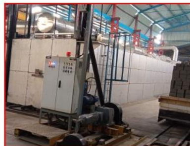
HIGH ALUMINA TUNNEL DRYER
