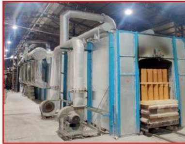
HIGH ALUMINA TUNNEL KILN
